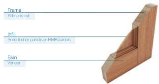
**solid construction doors** consist of a meranti or pine frame and door skin with a thick panel of solid MDF. This type of construction is most suitable for entrance door designs with routered patterns and glass openings.
