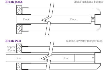
**Please note:** To convert a flush jamb cavity into a flush pull unit, install the  $2 \times 60$ mm converter bumper stops (included in the fittings) onto the back member as close as possible to the existing bumper stops. Some unit sizes/types may not be available in all states.
