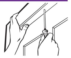
Screw in place the removable fillets using  $4 \times 35 \text{mm}$  countersunk screws through a white snap cap base. Finish off with supplied snap caps. Refer to drawing in step 12 and diagram 12A or 12B depending on your state.
