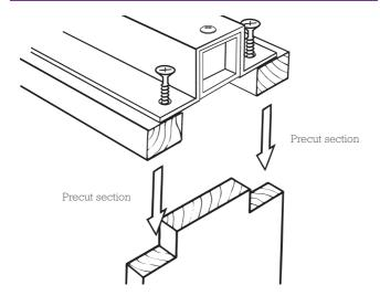
Cut down the sides from the end of the closing jamb – refer to the pre cut section in the detail shown. Screw/nail (not provided with fittings) the closing jamb to the head section fixing through the head timber into the closing jamb stile.
