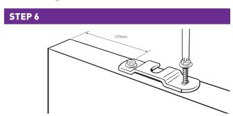
Attach the  $2\ x$  door support brackets to the top of the door using the  $4\ x$  30mm hex head screws, 100mm in from each side.
