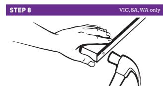
Cut the 2 x glide guide strips to suit the door width. Tack both strips to the bottom of the door using  $5\,\mathrm{x}$  panel pins with each glide guide strip. (total  $10\,\mathrm{x}$  panel pins).
