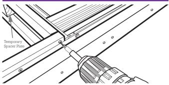
Fit and screw the head track assembly to the cavity pocket using the  $10\,\mathrm{x}$   $16\mathrm{mm}$  button head metal thread screws. Do not remove the temporary spacer plates in the opening of the cavity throat until the wall sheeting has been completed.
