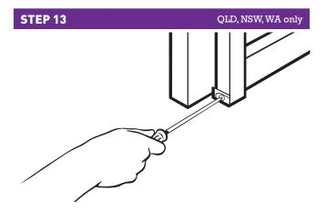
Fix the two nylon finger guides to the base of the frame using the elongated opening (for subsequent adjustment). The flexible portion protrudes into the cavity. When the guides are positioned correctly, fasten with  $2 \times 15 \text{mm}$  round head screws.
