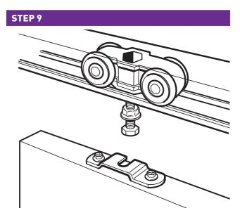
With the door in the opening, lift to locate each door support bracket onto the carriage assembly thread, ensuring the self locking nuts are above the bracket.
