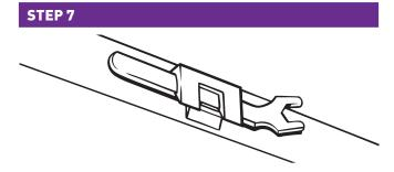
Attach the 1x spanner storage clip to the top of the door using the  $1 \times 15 \mathrm{mm}$  countersunk screw.
