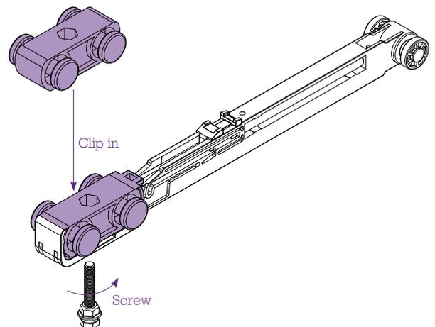
Take the bolt removed in step 3, screw the bolt through the soft closer and the trolley so that the door can be rehung.
