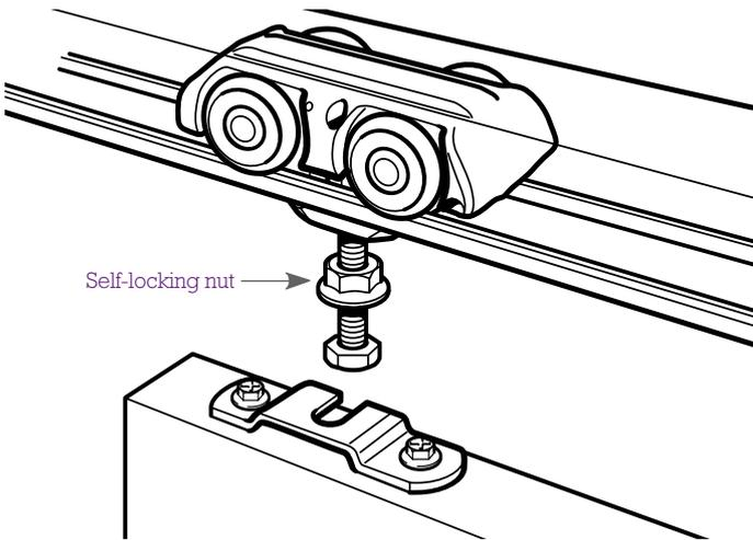
To unscrew the door from the trolley closest to the closing jamb, start by removing the removable fillets.
