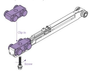
Take the bolt removed in step 2, screw the bolt through the Soft Closer and the trolley so that the door can be rehung.
