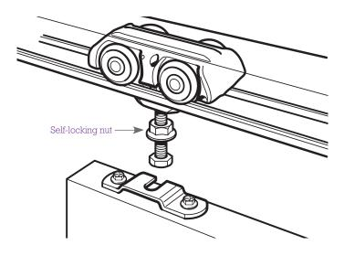
To unscrew the door from the trolley closest to the closing jamb, start by removing the removable fillets.
