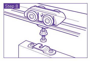
Step 8. With the door in the opening, lift to locate each door support bracket onto the carriage assembly thread, ensuring the self locking nuts are above the bracket.
