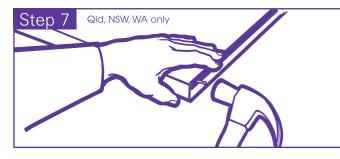
Step 7. Cut the 2 glide guide strips to suit the door width. Tack both strips to the bottom of the door using 5 panel pins with each glide guide strip.
