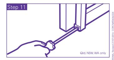
Step 11. Fix the two nylon finger guides to the base of the frame using the elongated opening (for subsequent adjustment). The flexible portion protrudes into the cavity. When the guides are positioned correctly, fasten with a 15mm round head fixing screw.
